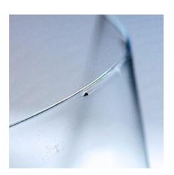
Extruded polymerfilm with visible defects
